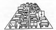
Level of Service F describes forced low operations after density has exceeded optimum which is normally in the range of 70 to 75 vpm on the free flowing facilities. Speed and rate of flow are below the levels attained in the zone E and may, for short time periods, drop to zero.
