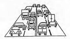
The upper limit of Level of Service E is the capacity of the facility. Operation in this zone is unstable, speeds and flow rates fluctuate, and there is little independence of speed selection or ability to maneuver. Since headways are short and operating speeds subject to rapid fluctuation, driving comfort is low and accident potential high. Although circumstances may make operation of facilities under these conditions necessary, it is clearly undesirable and should be avoided wherever feasible.
