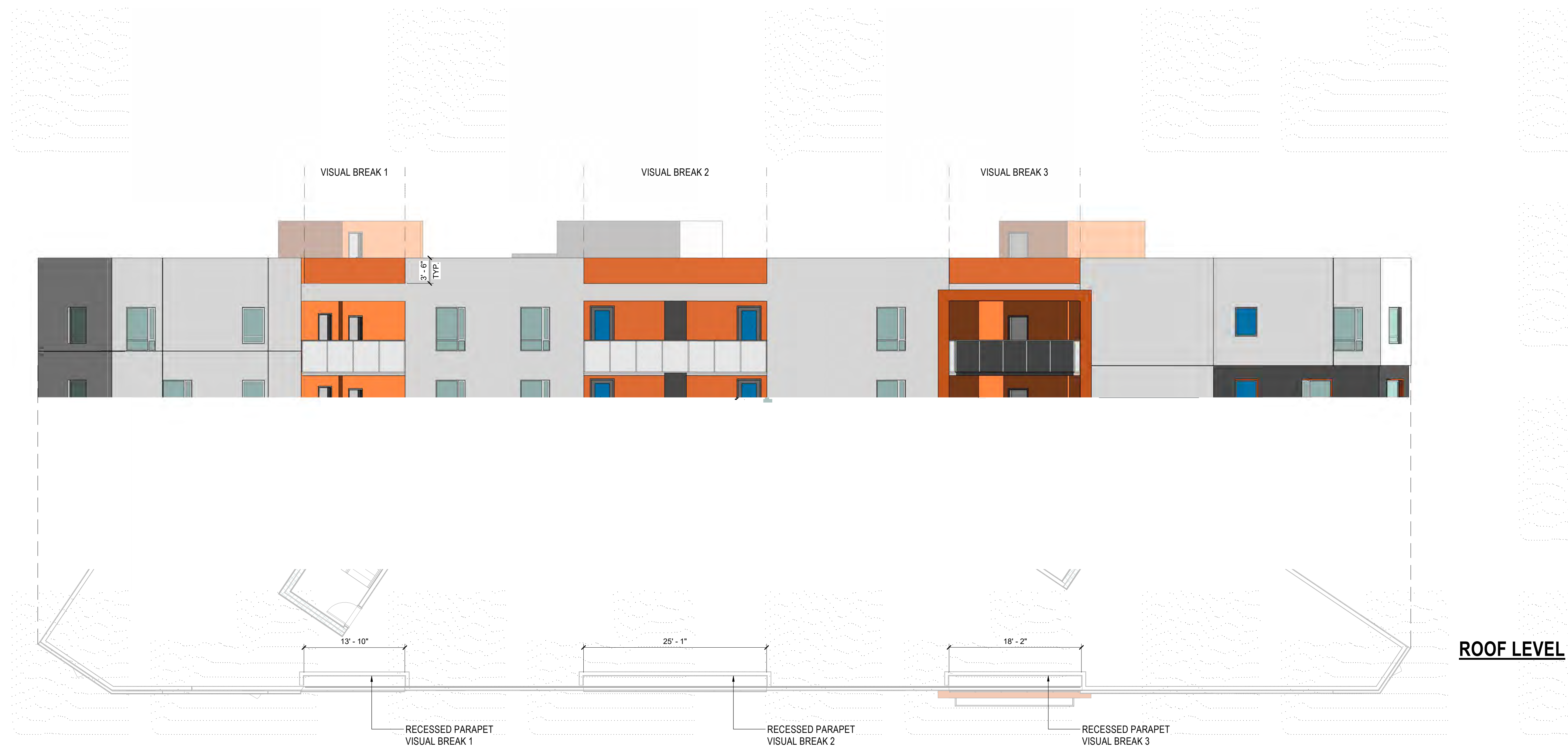
1 ROOF VISUAL BREAK DIAGRAM 1/8" = 1'-0"
