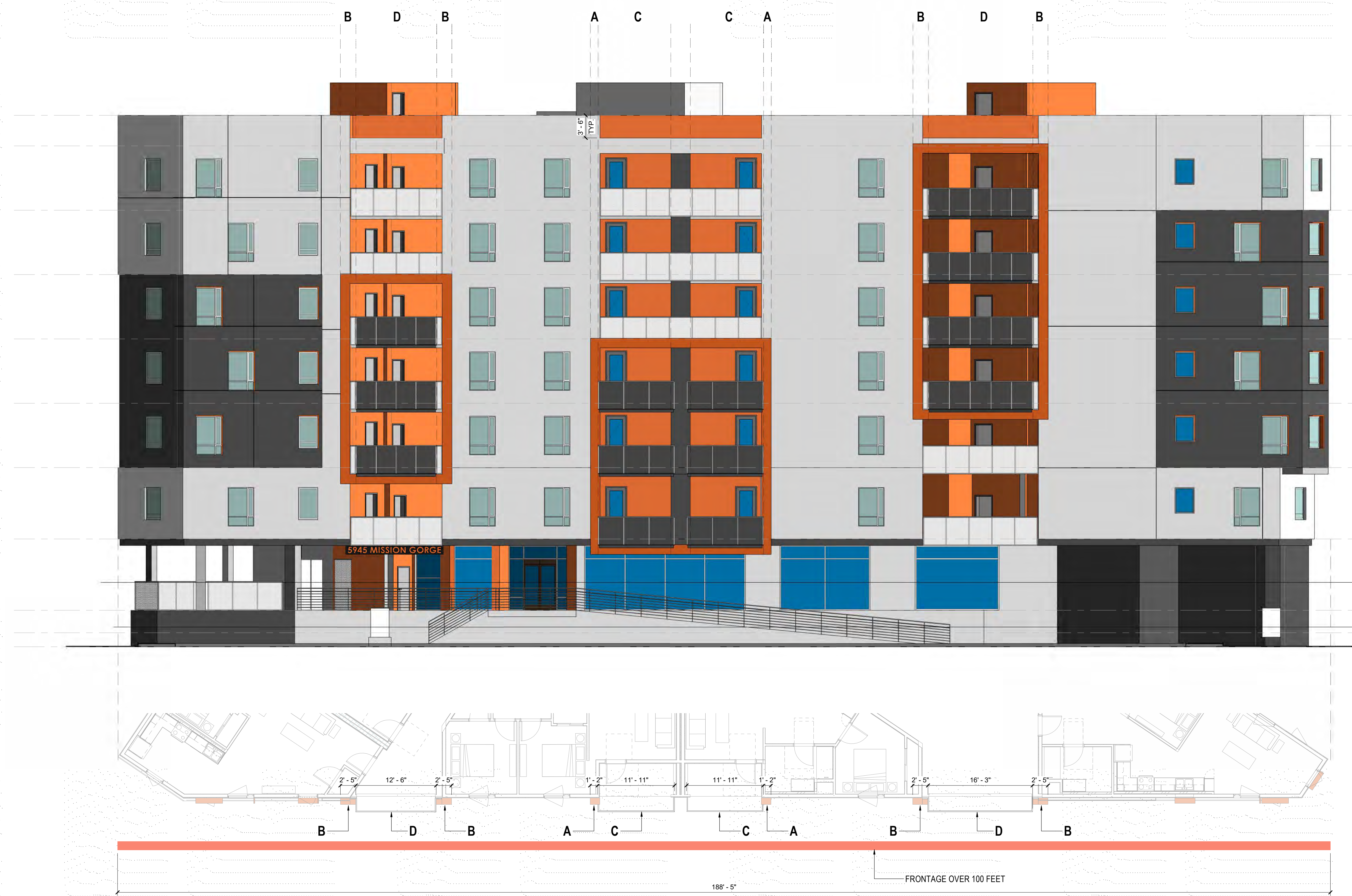
1 OFFSETTING PLANES DIAGRAM 1/8" = 1'-0"
