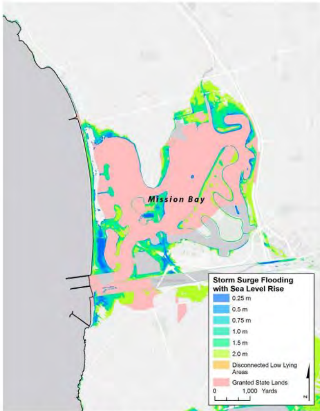
Figure 3. Mission Bay exposure to storm surge and sea level rise.
