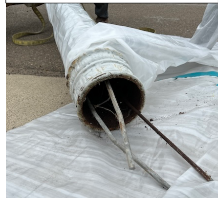
Top of anchor rods and internal assembly rods not accessible due to soldered connection at collar.
