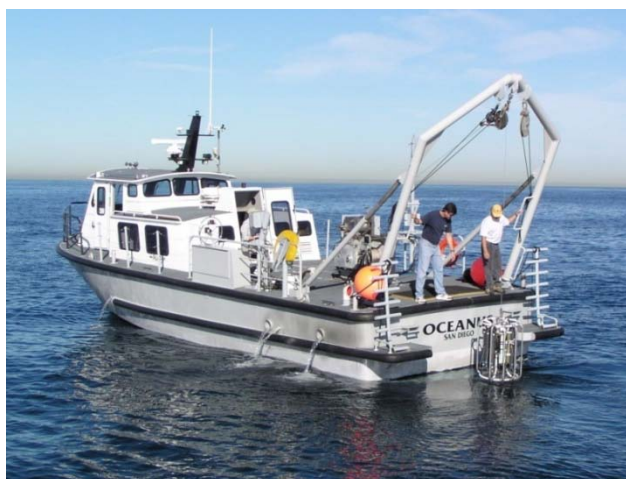
To ensure protection of San Diego's ocean environment, the City of San Diego monitoring program maintains two ocean monitoring vessels which operate offshore a combined total of approximately 200 days each year collecting water quality, sediment, benthic, and trawl samples. The 48-foot Oceanus is shown above.
