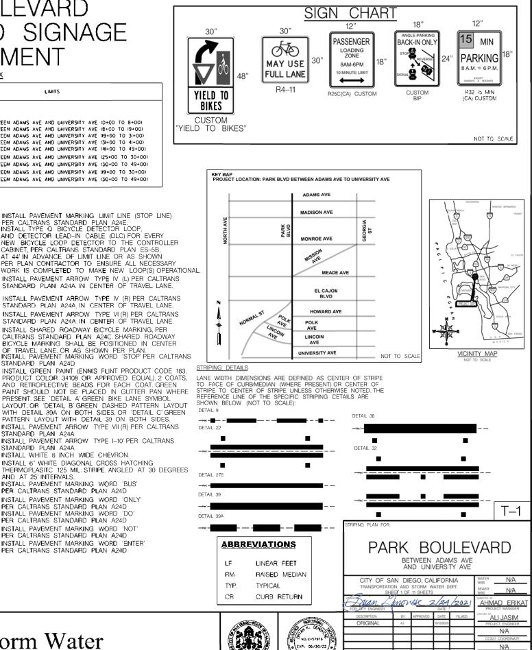
8 INSTALL PAVEMENT ARROW TYPE IV (R) PER CALTRANS STANDARD PLAN A24A, IN CENTER OF TRAVEL LANE.
