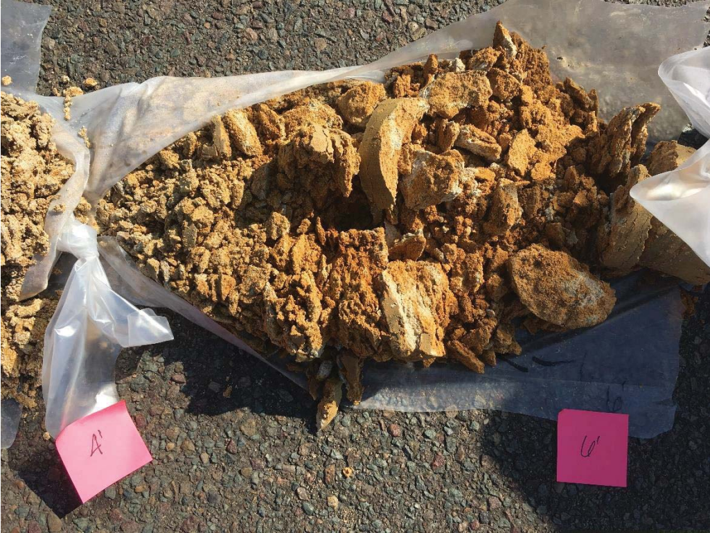
Figure 1. Boring B-1 Sample from 4 to 6 Feet Below Ground Surface.
