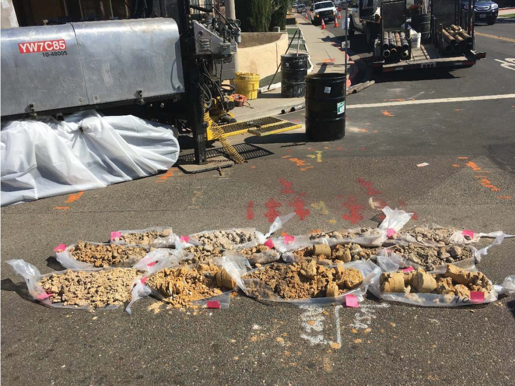
Figure 7. Boring B-1 Samples from 2.5 to 30 Feet Below Ground Surface.
