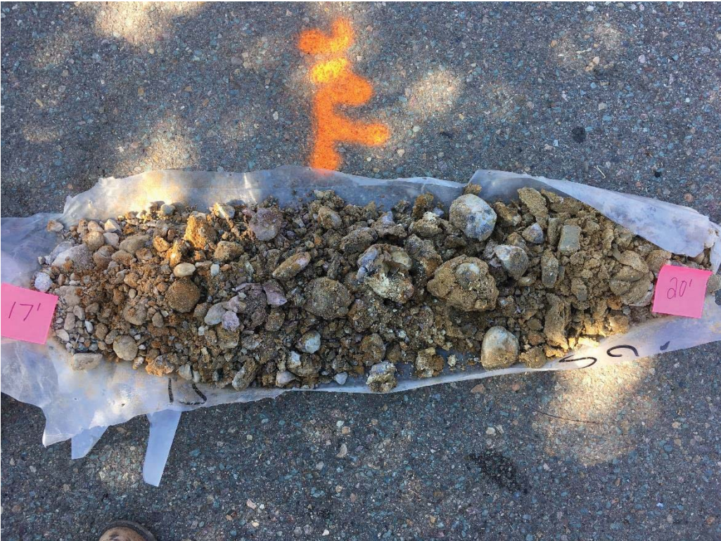
Figure 10. Boring B-2 Sample from 17 to 20 Feet Below Ground Surface.
