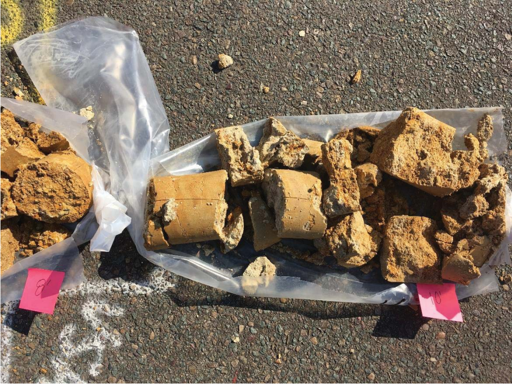
Figure 2. Boring B-1 Sample from 8 to 10 Feet Below Ground Surface.
