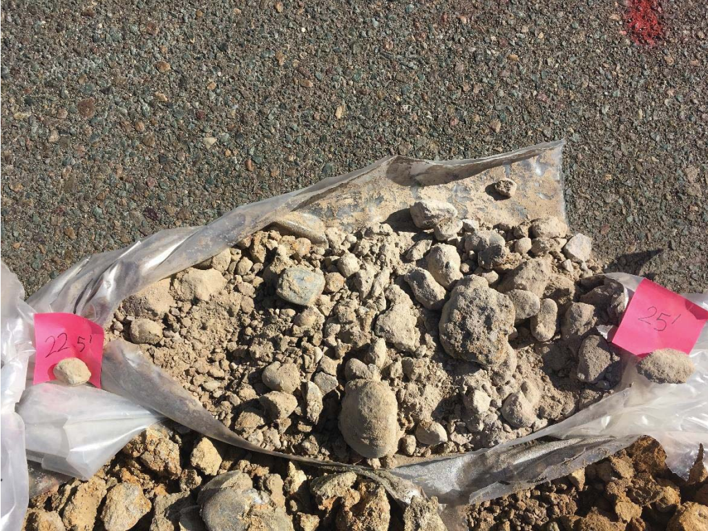
Figure 5. Boring B-1 Sample from 22.5 to 25 Feet Below Ground Surface.
