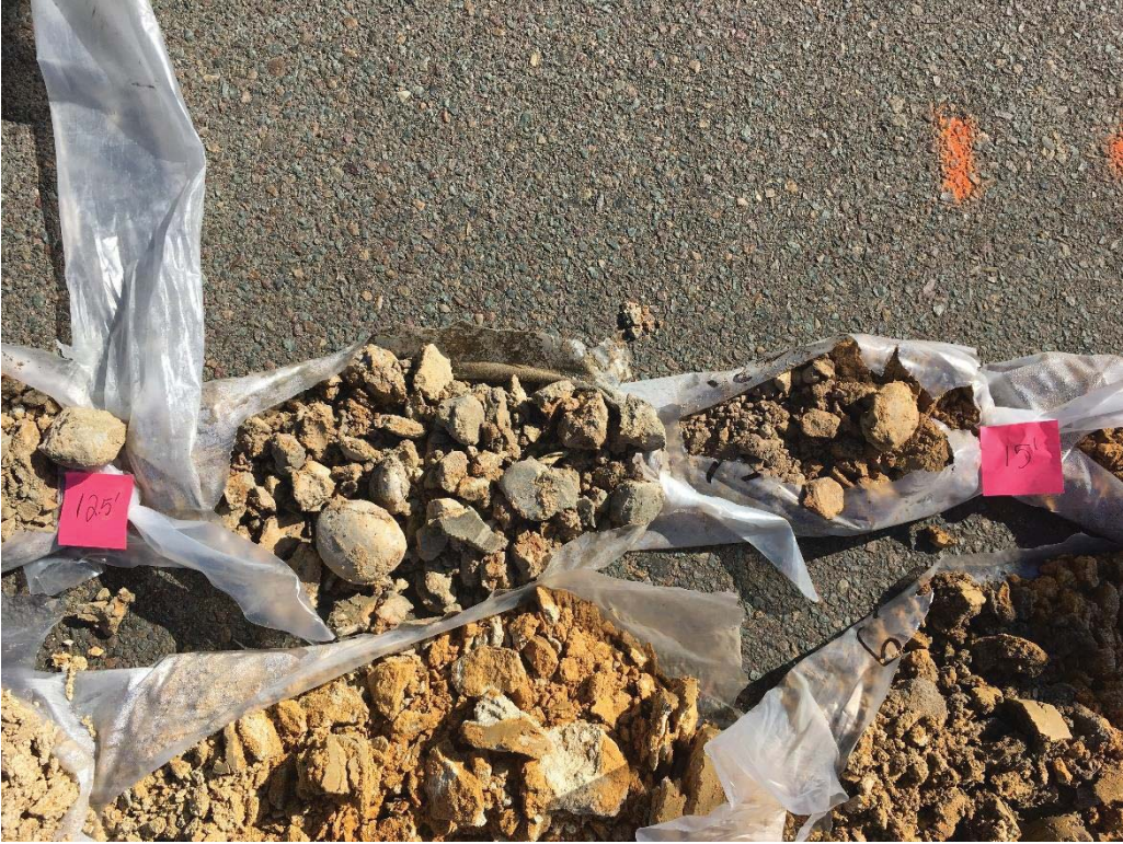
Figure 3. Boring B-1 Sample from 12.5 to 15 Feet Below Ground Surface.
