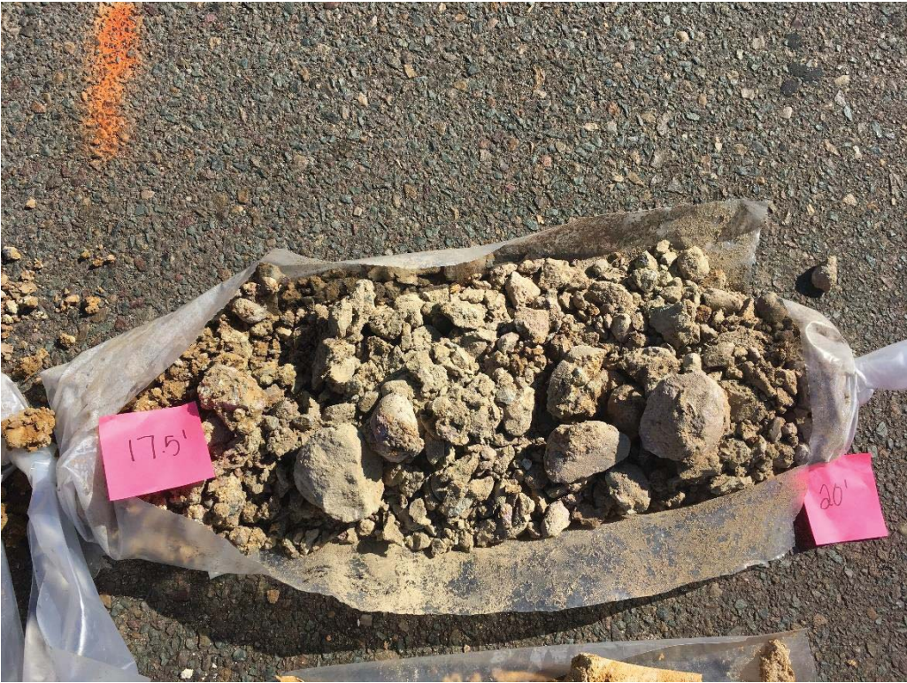
Figure 4. Boring B-1 Sample from 17.5 to 20 Feet Below Ground Surface.
