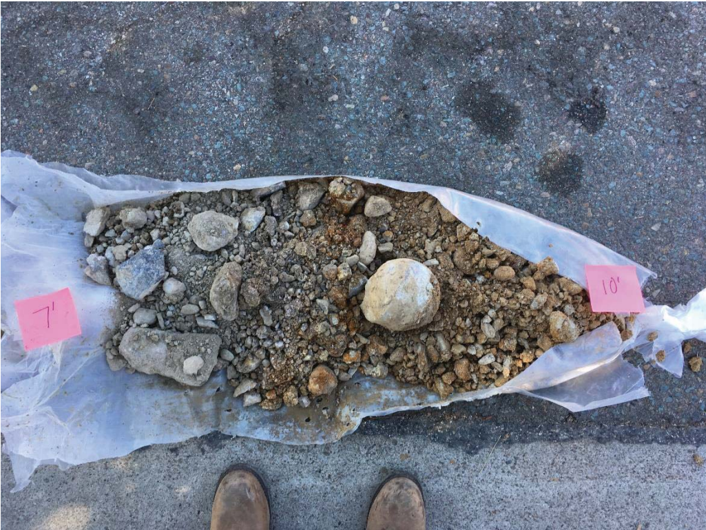
Figure 8. Boring B-2 Sample from 7 to 10 Feet Below Ground Surface.
