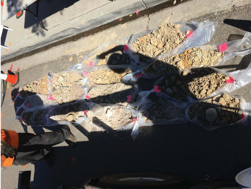
Figure 15. Boring B-2 Sample from 5 to 40 Feet Below Ground Surface.
