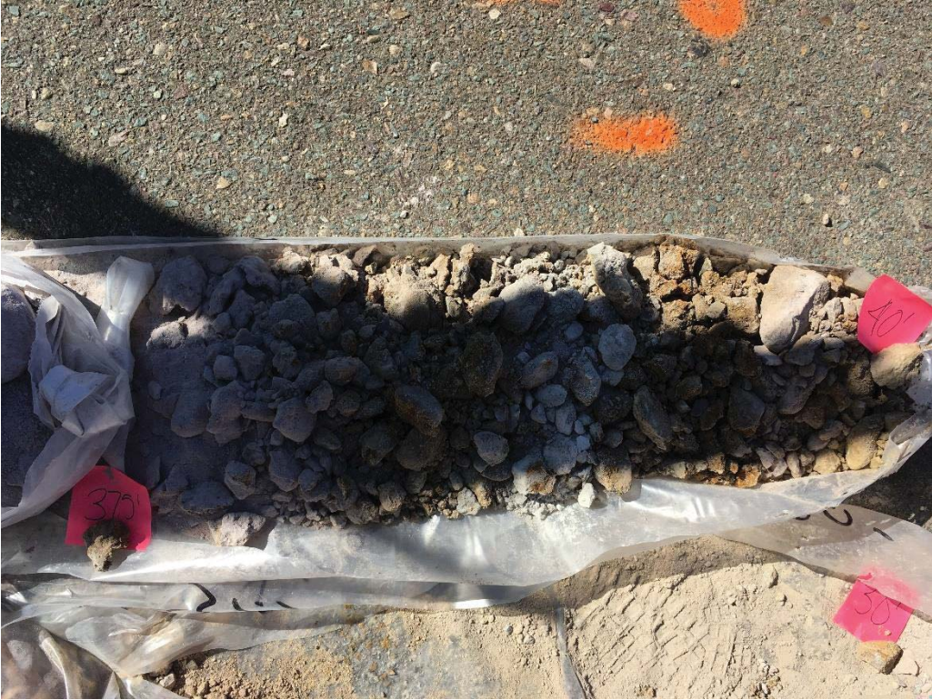
Figure 14. Boring B-2 Sample from 37.5 to 40 Feet Below Ground Surface.
