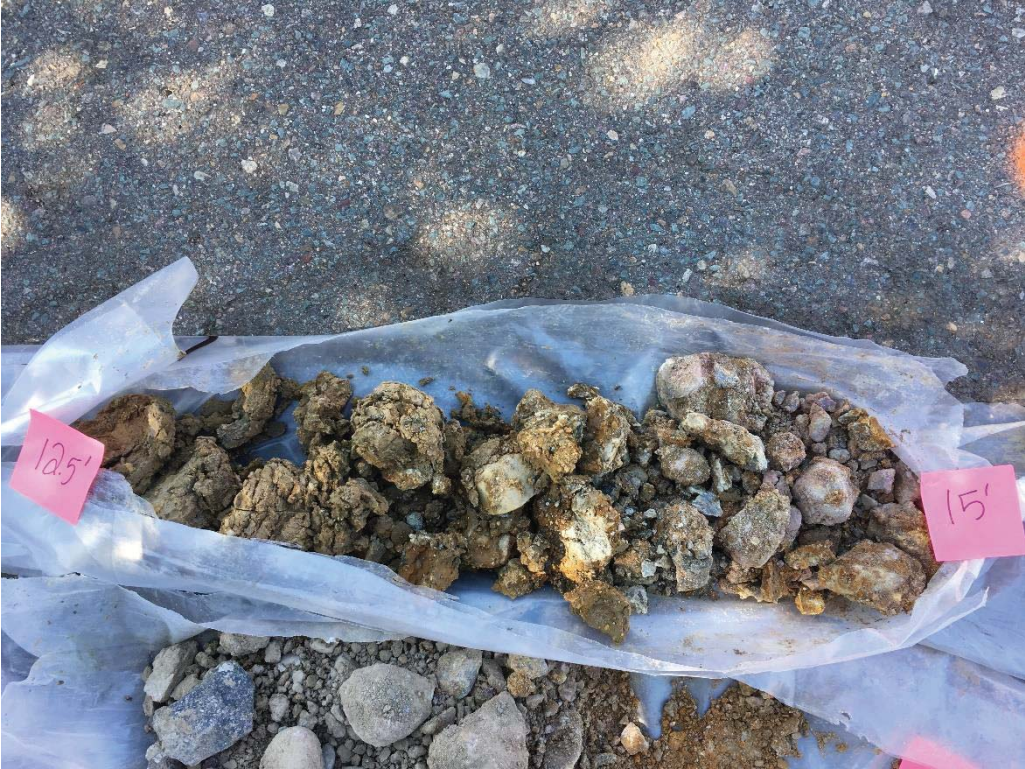
Figure 9. Boring B-2 Sample from 12.5 to 15 Feet Below Ground Surface.
