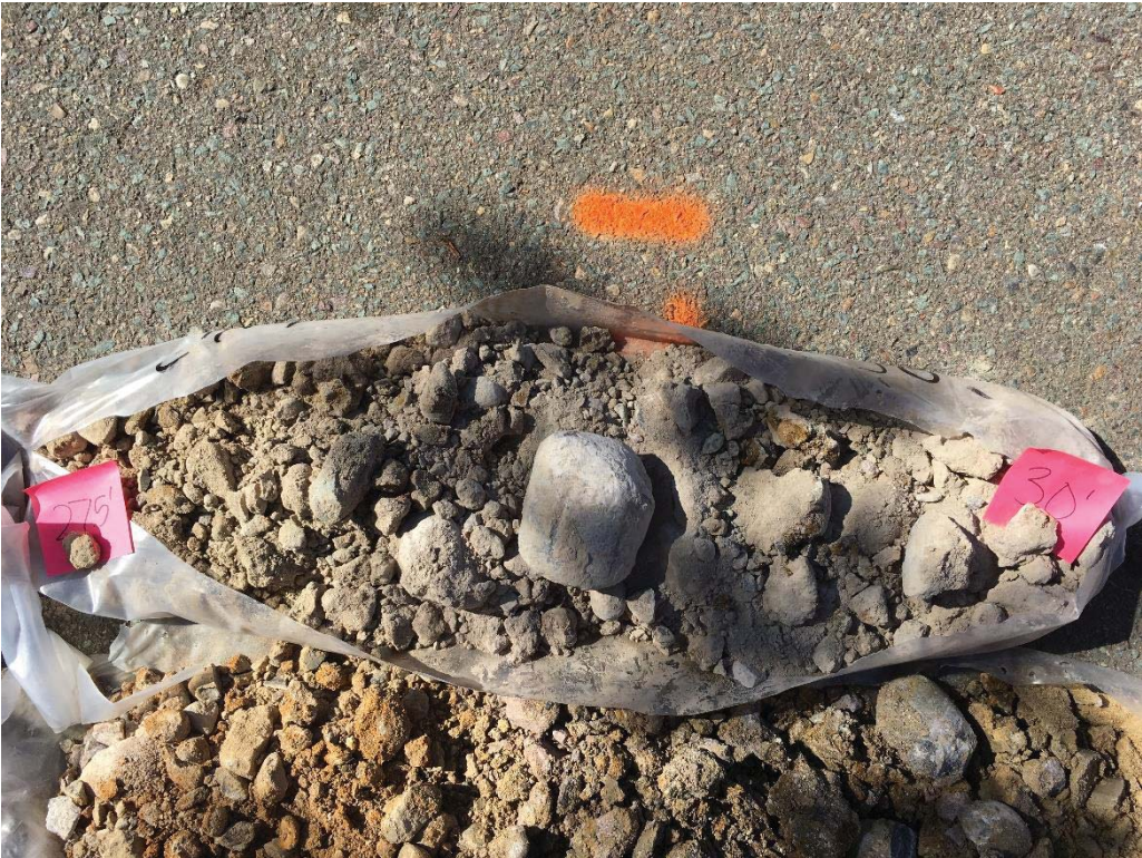
Figure 12. Boring B-2 Sample from 27.5 to 30 Feet Below Ground Surface.
