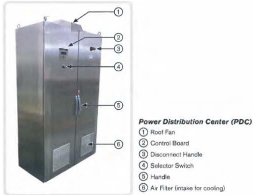
Figure 73. Power Distribution Center
