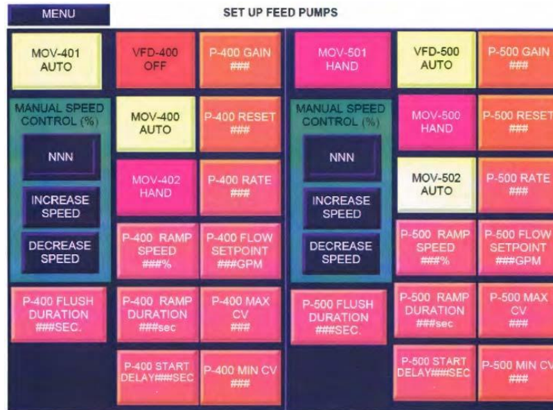
Figure 63. Feed Pump Operating Parameter Entry Screen
