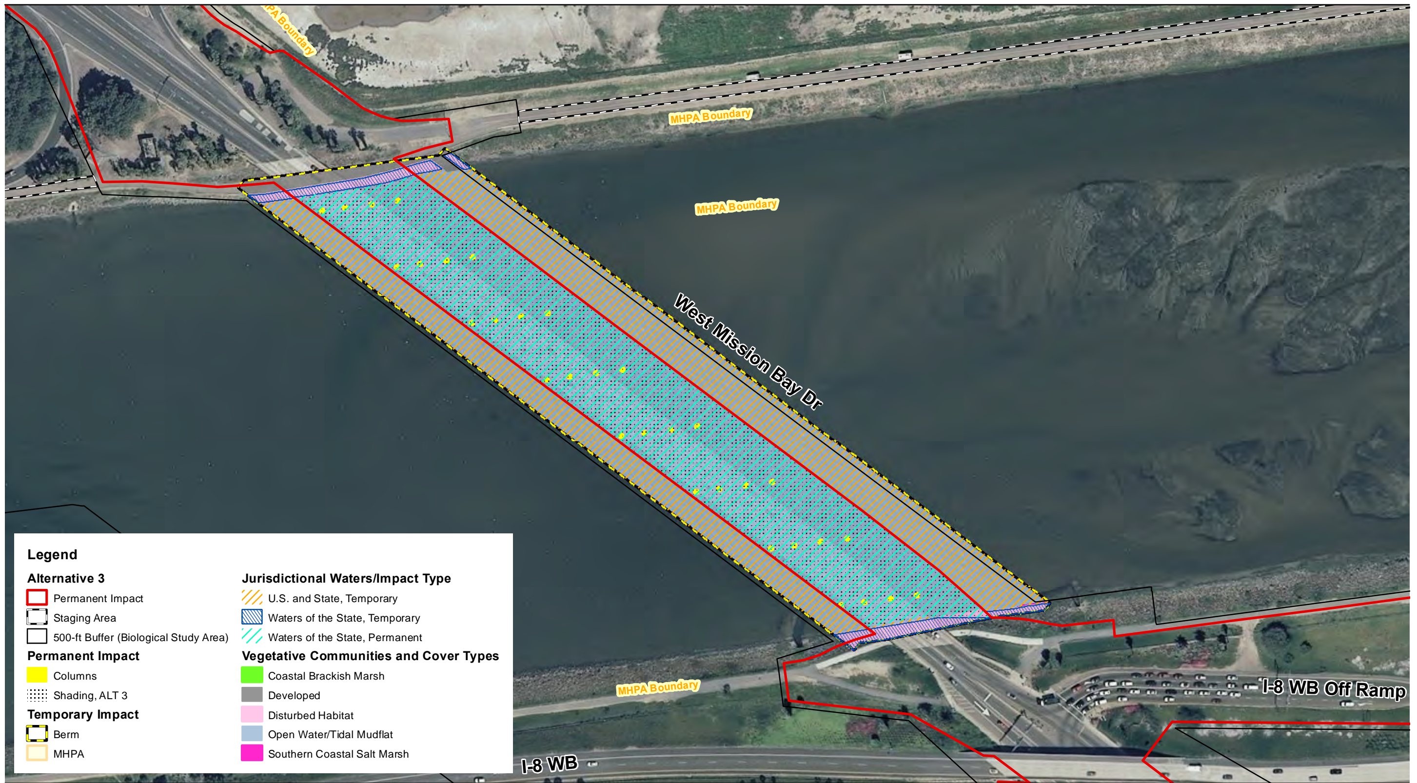
Figure 2.3.10-5 Alternative 3 – Potential Impacts to Waters of the U.S. and State Related to Construction of Temporary Large Berm
