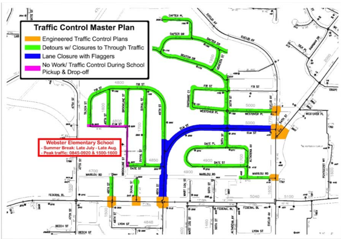
Figure 4 – Traffic Control Master Plan
