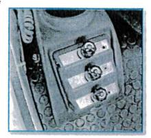
Adjusting valve is mounted on the outside, near the nozzles installed on the extraction hose end / container inlet, for works that are carried out in particularly dusty places.
