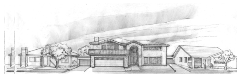
“Inappropriate in-fill due to building proportions and garage placement.”
