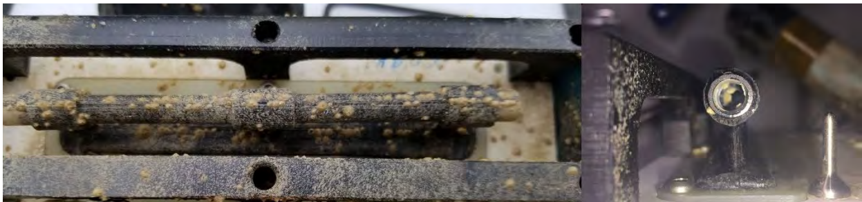
Figure 2: Cell with newly spawned barnacles; requires cleaning
