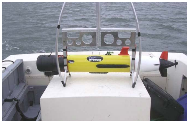
Figure 5. REMUS vehicle on boat prior to mission deployment (GPS, sidescan sonar, ADCP, CTD, backscatter, colored dissolved organic matter [CDOM]).
