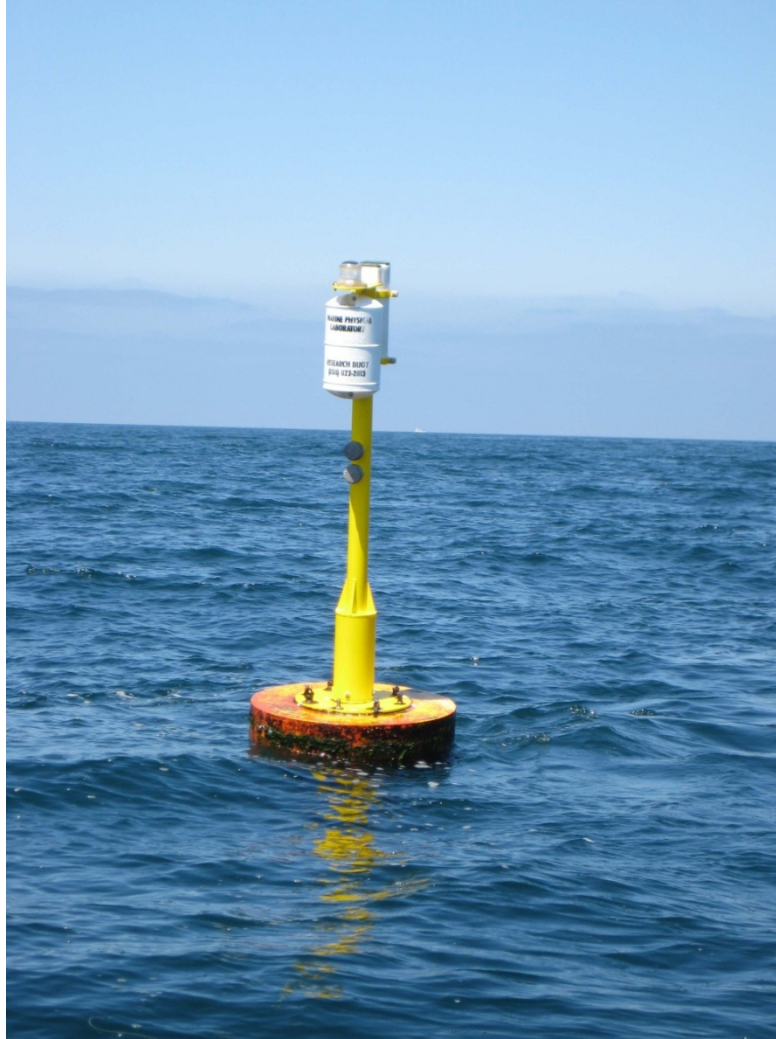
Figure 3. Photograph of the deployed ocean buoy at the PLOO. The white cylinder on the right is a radar reflector and the cylinder on the left is a GPS tracking device.
